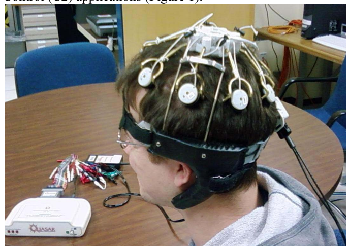
Figure 1. The prototype QUASAR dry electrode system for electroencephalographic recording.
