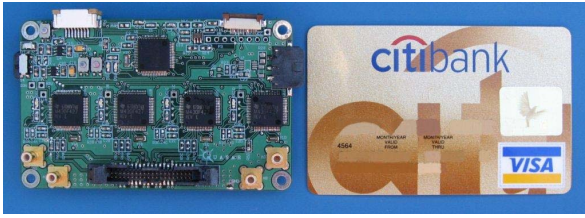
Fig. 3 Prototype Data Acquisition board with credit card for scale.
