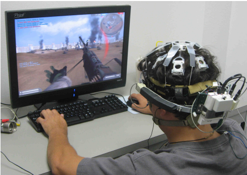
Fig. 7. A test system for assessing workload and engagement of computer gamers.
