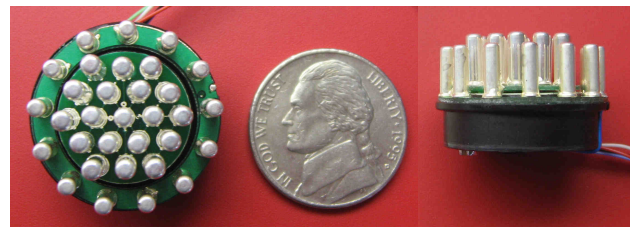
Fig. 1. QUASAR hybrid EEG biosensor (with a US 5 cent coin for scale).
