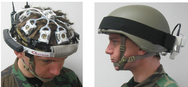
Fig. 2. Hybrid sensor array incorporated into a soldier's Kevlar helmet. Left: The outer aluminium ring and weights load the harness correctly when the helmet is not present. Right: EEG system with helmet attached and ready for use, including wireless module.
