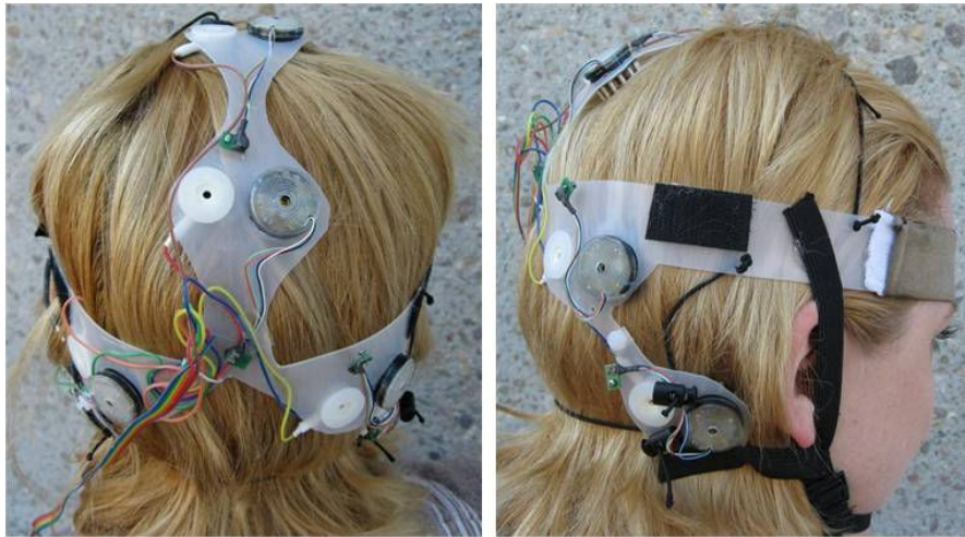
Fig. 3. Headpiece used to make simultaneous HESA and WEA electrode comparison measurements. Spring loaded clamps on the elastic pieces made for quick and convenient adjustment for head size and sensor loading. The smaller electrodes on the left (right panel) are the WEA electrodes, and the larger disk to the right is the HESA electrode.
